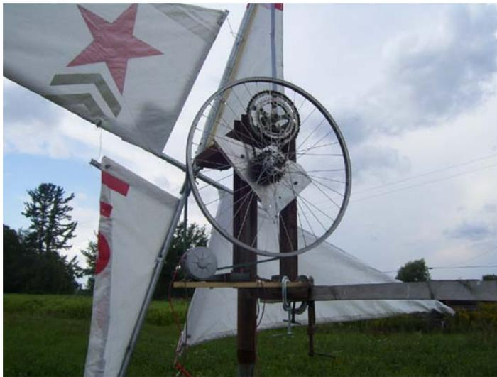
The second is to create the wings or four branches of the rotor from a low cost replaceable material, if possible one which detaches itself in strong wind without destroying not only the steel structure but also the wings. Here we are finding the inspiration from sailboating, using a set of sails or jibs controlled by a simple system of releasing cables or strings.
