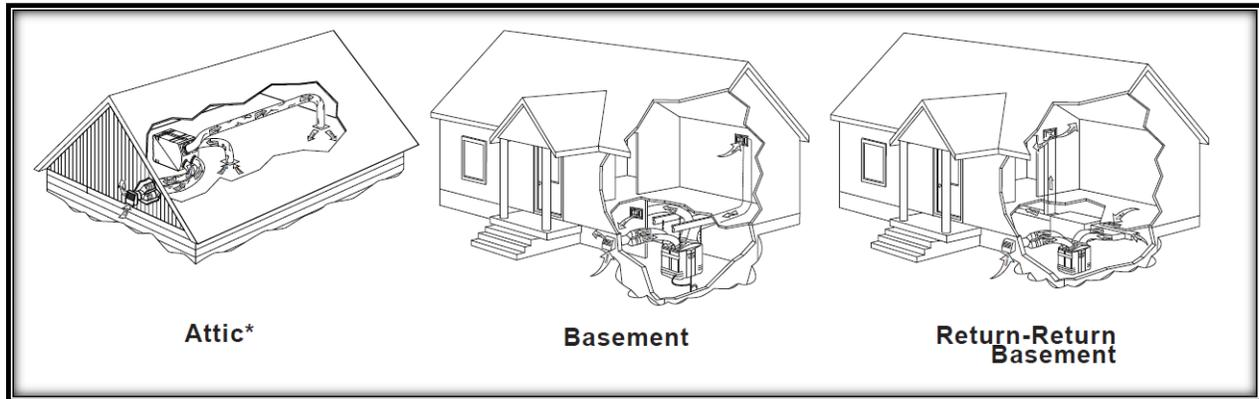
Figure 55 Example installation setups for the Broan HRV system (Appendix C)
