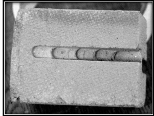
Figure 52 Example of the sampling technique used by University of Bath for a 50mm wide lime wall specimen.
