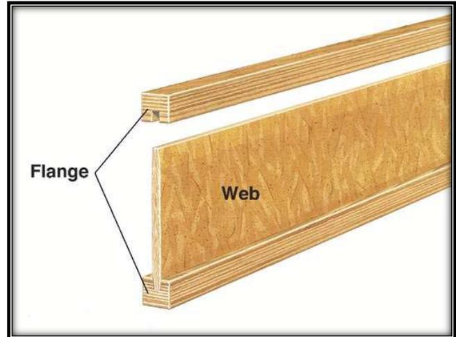
Figure 57 I-Joist Cross Section
