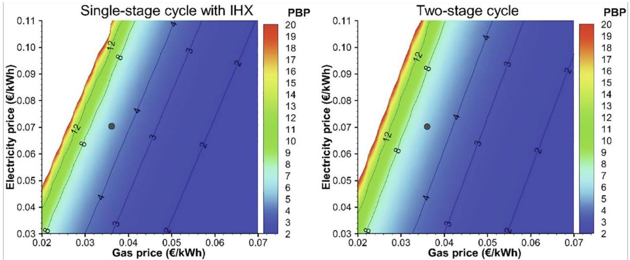
Figures 2 & 3: Discounted payback period of a single-stage heat pump with an internal heat exchanger and a two-stage heat pump.
