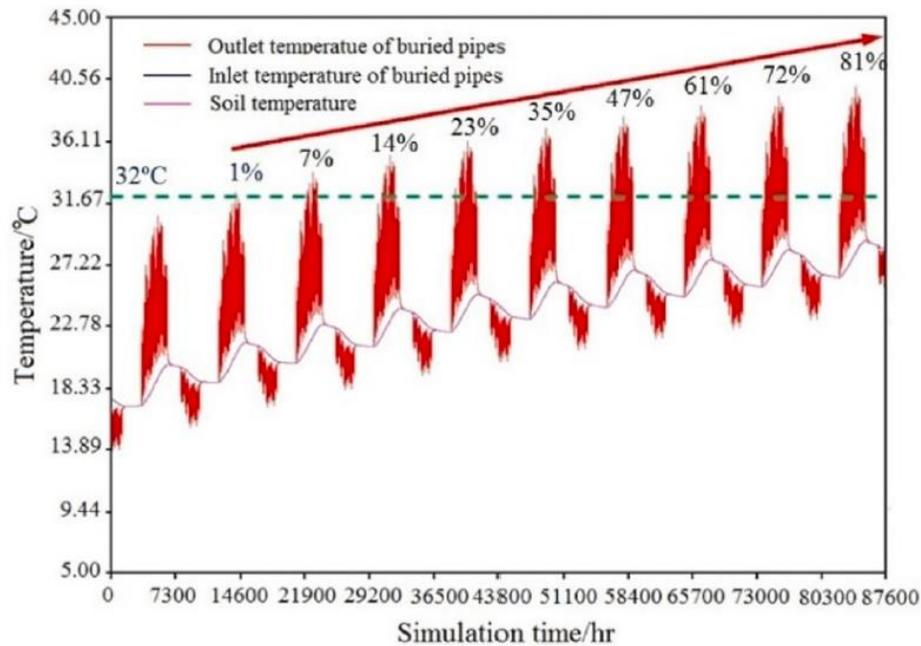
Figure 15. Soil Temperature Increases as the GSHP Works (Xu et al., 2021)
