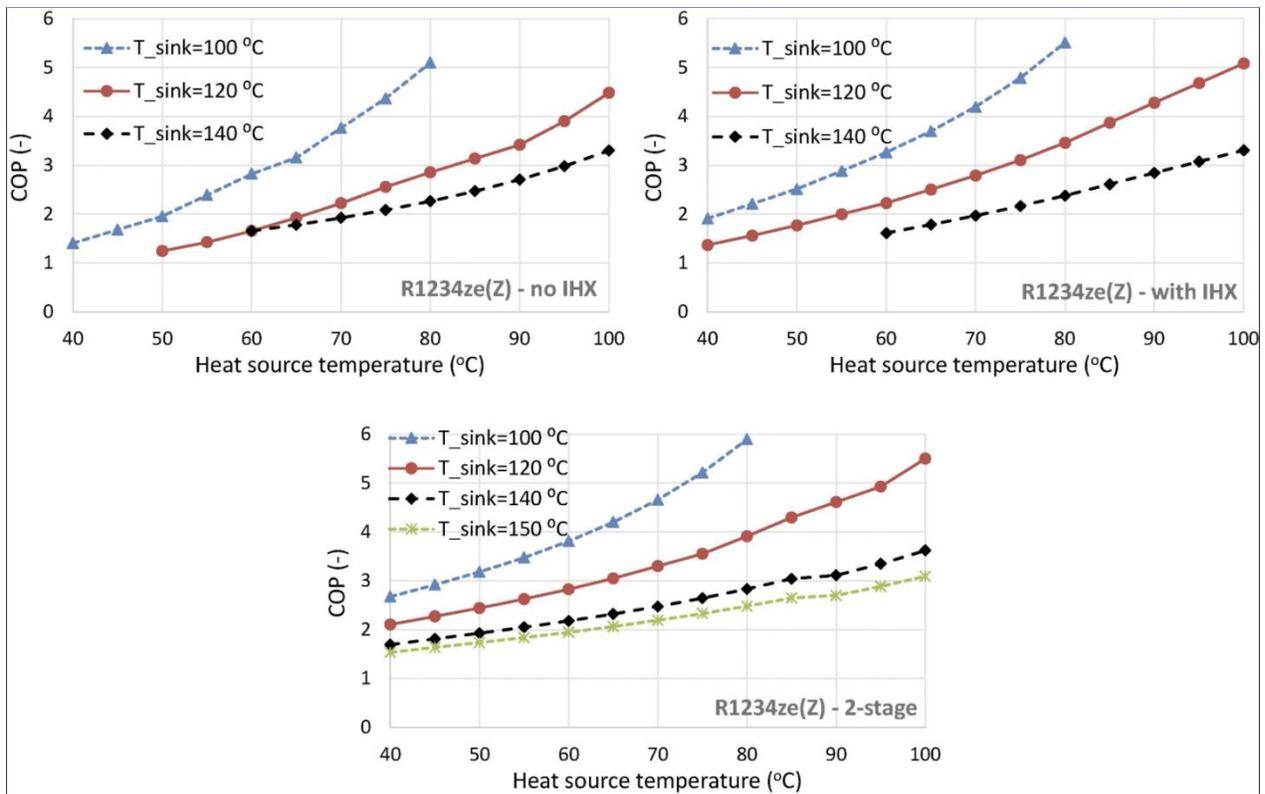
Figure 1: COP of single-stage, single-stage with internal heat exchanger, and two-stage heat pump configurations (Kosmadakis, et. al. 2020).
