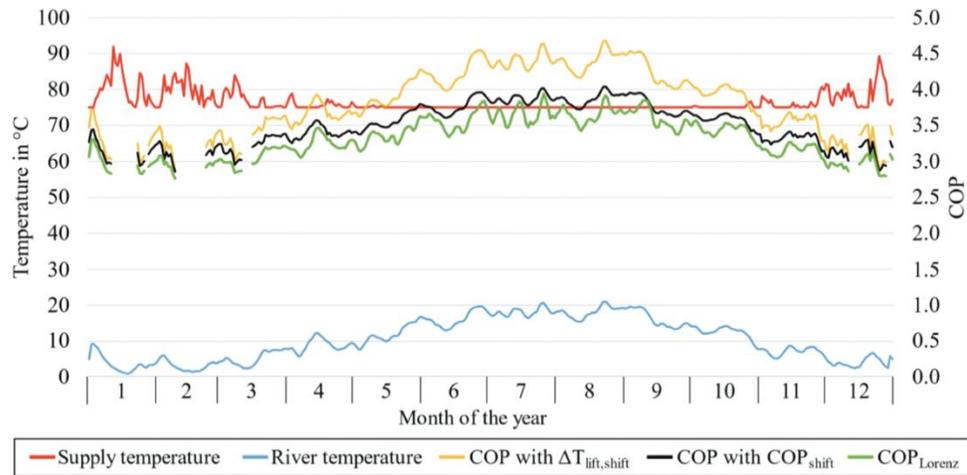
Figure 5: COP vs. time by modeling methodology (Trabert, et. al. 2021)
