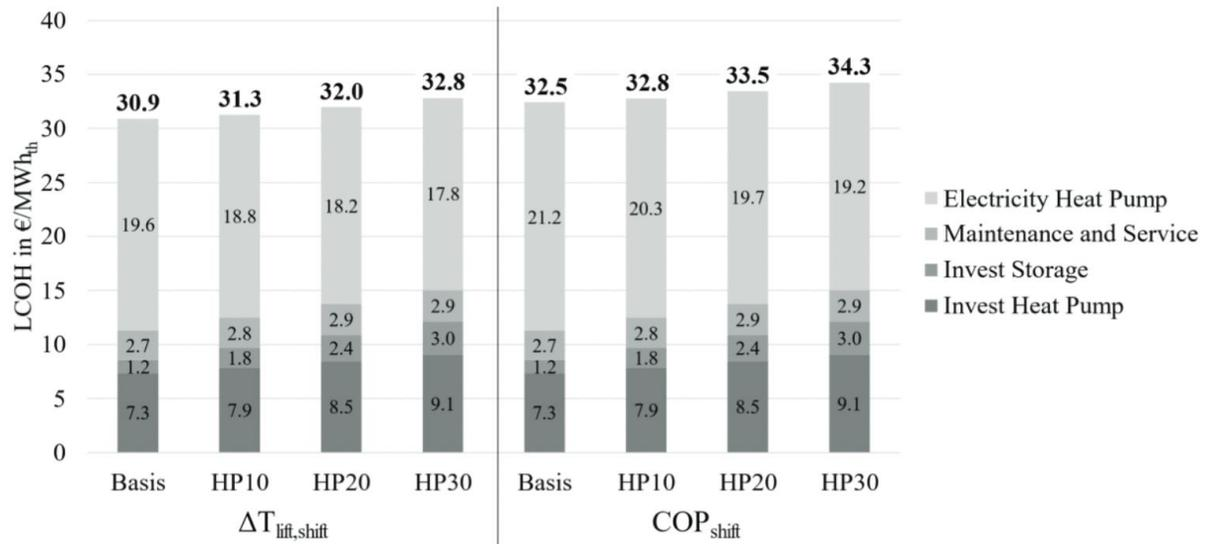
Figure 6: Comparison of LCOH of 4 different heat pump and storage size scenarios and 2 different modeling methodologies.
