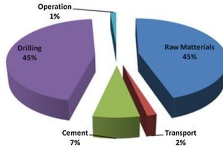
Figure 14: NOx Emissions from all Stages during the GSHP System Life Span (Koroneos & Nanaki, 2016)
