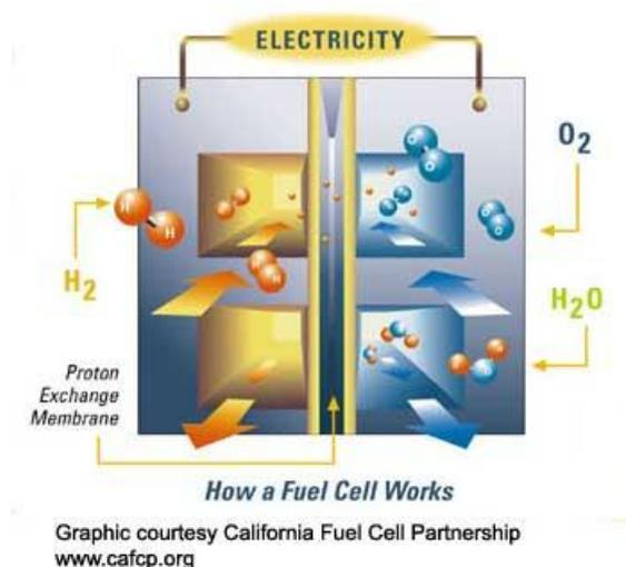
**Figure 4.1.** Diagram of a fuel cell. Reference: Detail of a hydrogen fuel cell, “Hydrogen fuel cell vehicles”, Electronic reference, Dream Green, [http://dream-green.org/wiki/index.php5?title=Hydrogen\\_fuel\\_cell\\_vehicles](http://dream-green.org/wiki/index.php5?title=Hydrogen_fuel_cell_vehicles), 02/15/2013.
