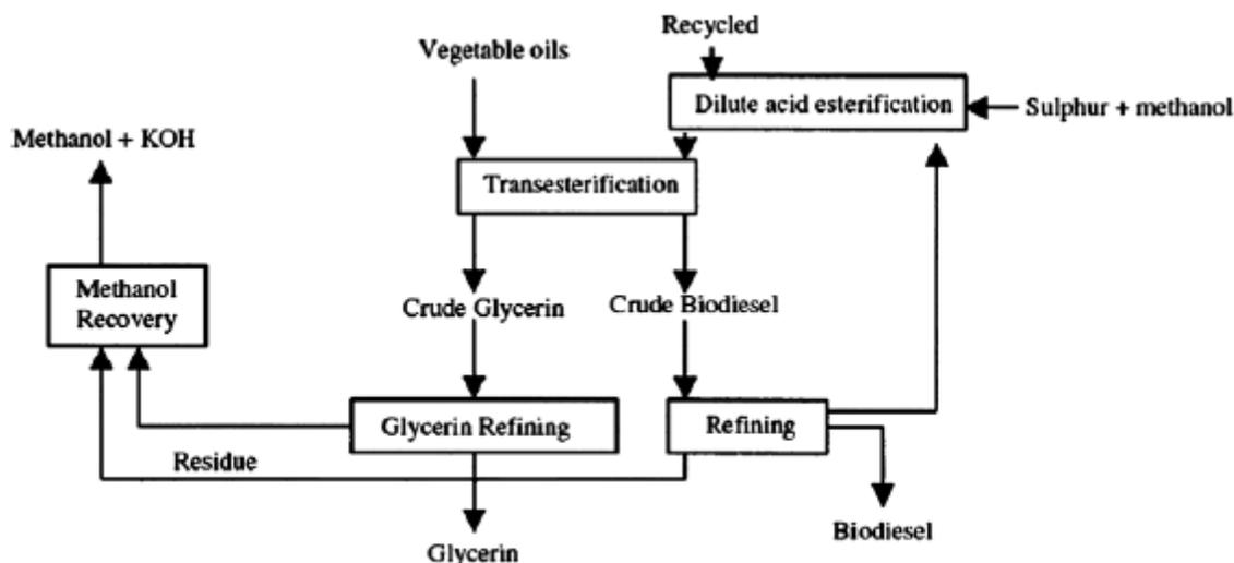
Fig. 1. Basic scheme for biodiesel production.
