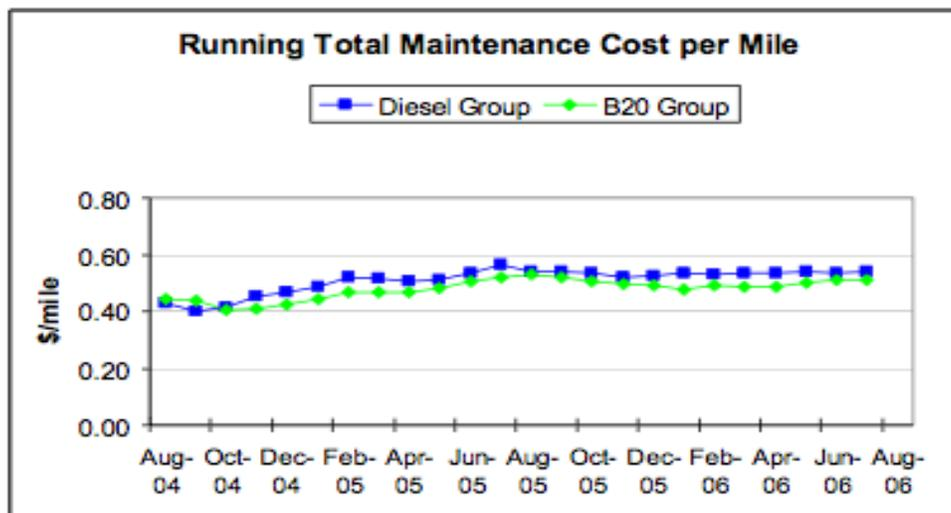
**Figure 1.8:** 100,000-Mile Evaluation of Transit Buses Operated on Biodiesel Blends.
