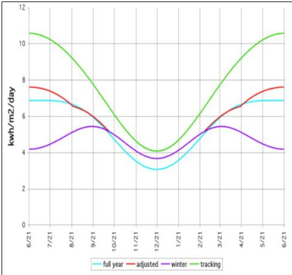
Fig. 3.2.c Effect of adjusting the angle (Landau,2017)
