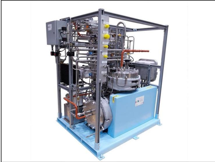
Figure 6.2. Two stage PDC-13 compressor
