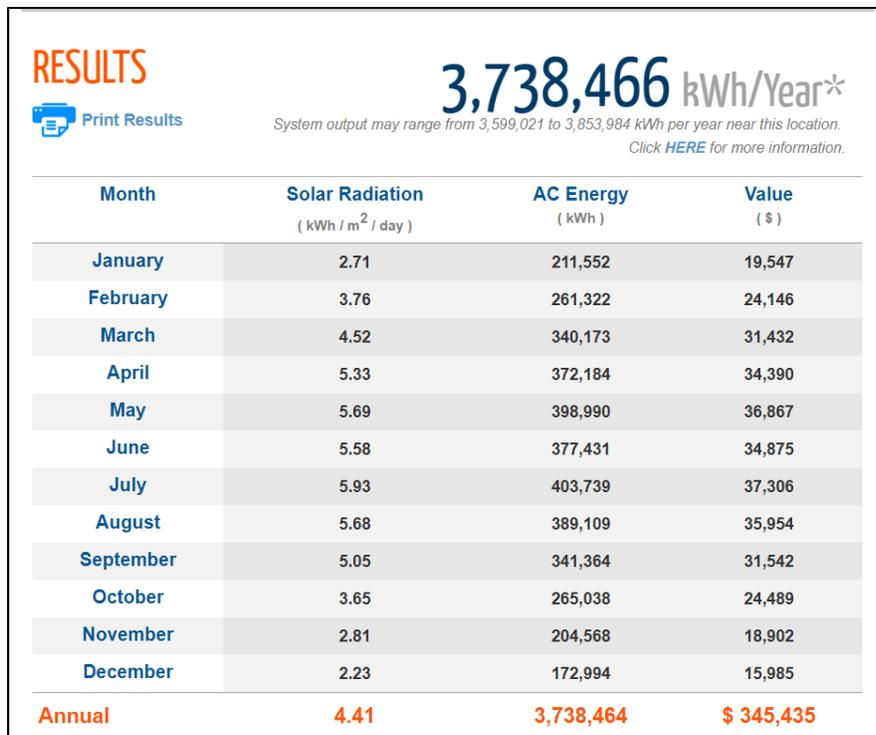
Fig. 3.2.f. 3MW system summertime Energy results (PVWatts , NREL)
