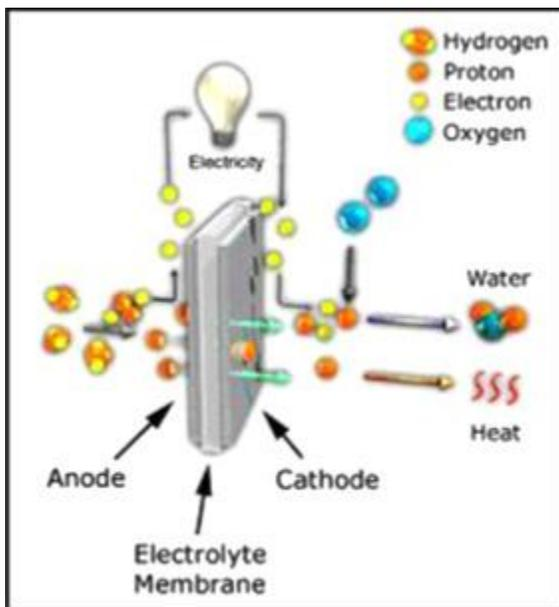
Fig. a. The mechanism of hydrogen fuel cell (Sharaf, )
