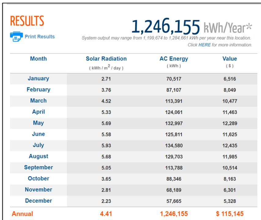
Fig. 3.2.g 1MW System Energy results (PVWatts , NREL)
