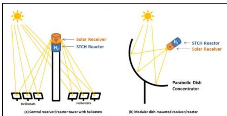
Figure 2.3.d Thermochemical water splitting
