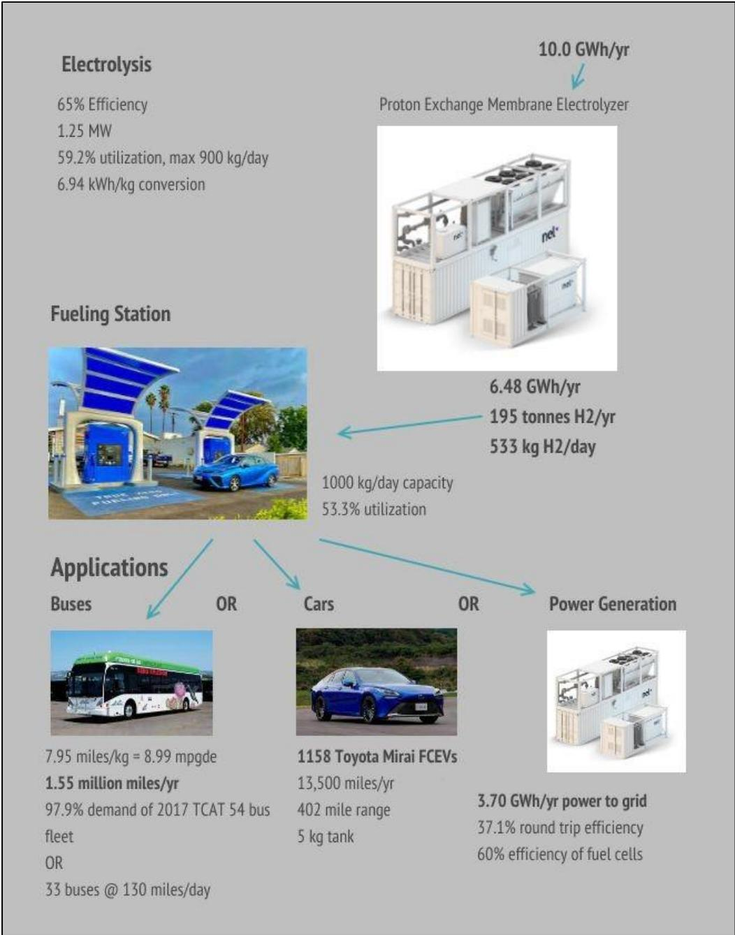
The model presented above aims to highlight the components of the production process for green hydrogen and estimate output that would be achievable with modern technology capabilities. The assumptions and model in full can be viewed in Appendix B. Detailed explanations of the reasons for the choices of assumptions for each of the components can be found in greater detail in each of the corresponding sections.
