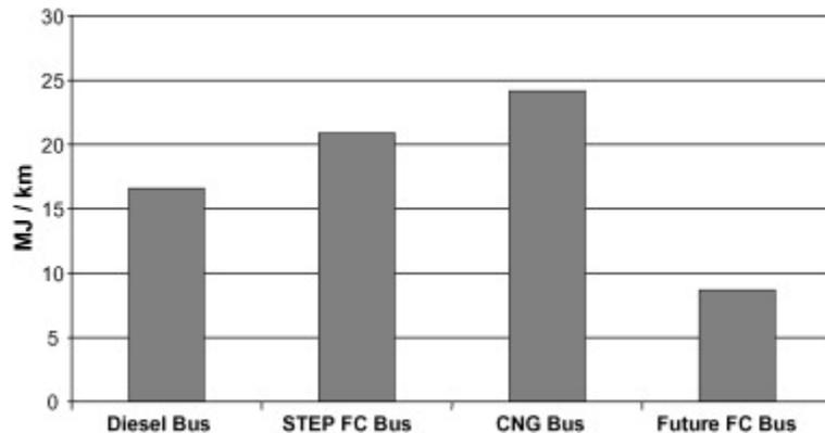
Fig. b. Comparison of vehicle energy efficiency for diesel, natural gas, hydrogen fuel cell, and future hydrogen fuel cell buses. (Ally, 2007).
