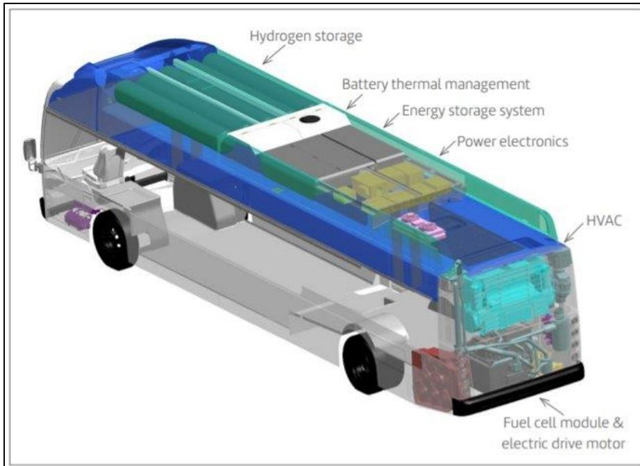
Figure 9.1 key components of hydrogen fuel cell bus
