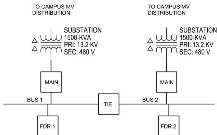
Figure 2.4.3 – Typical Building Distribution with Main-Tie-Main Configuration
