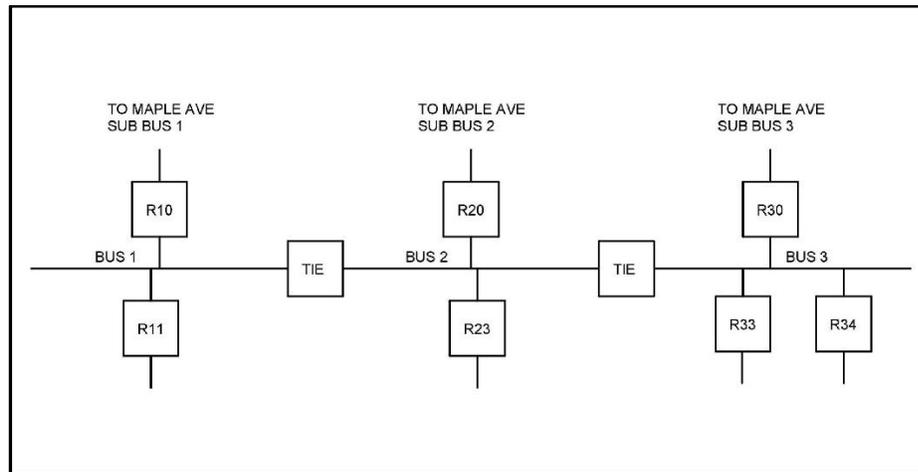
Figure 3.4A – Campus Road Substation Bus Configuration
