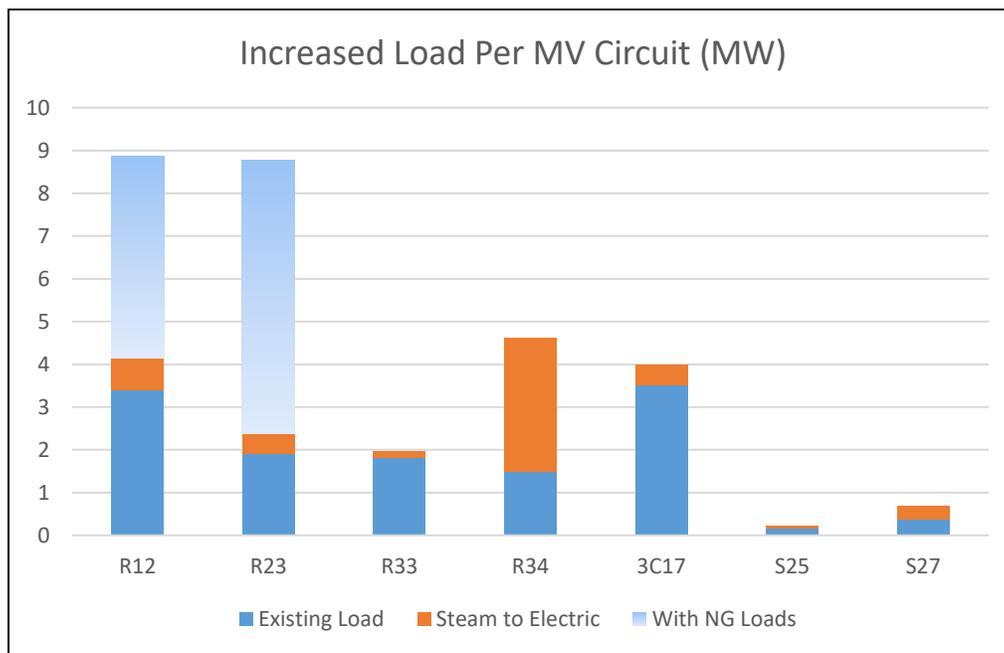
Figure 3.4.2 – MV Circuit Load Increases with NG Loads Included
