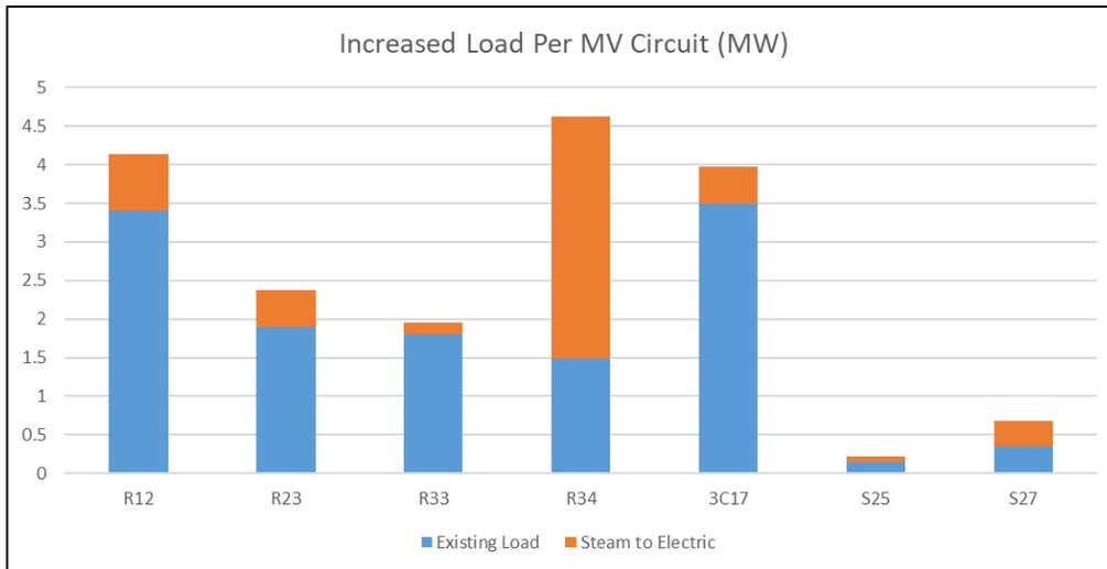
Figure 3.4I – Proposed Additional Load on MV Circuits
