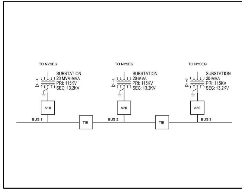
Figure 1.3 Campus Substation Configuration
