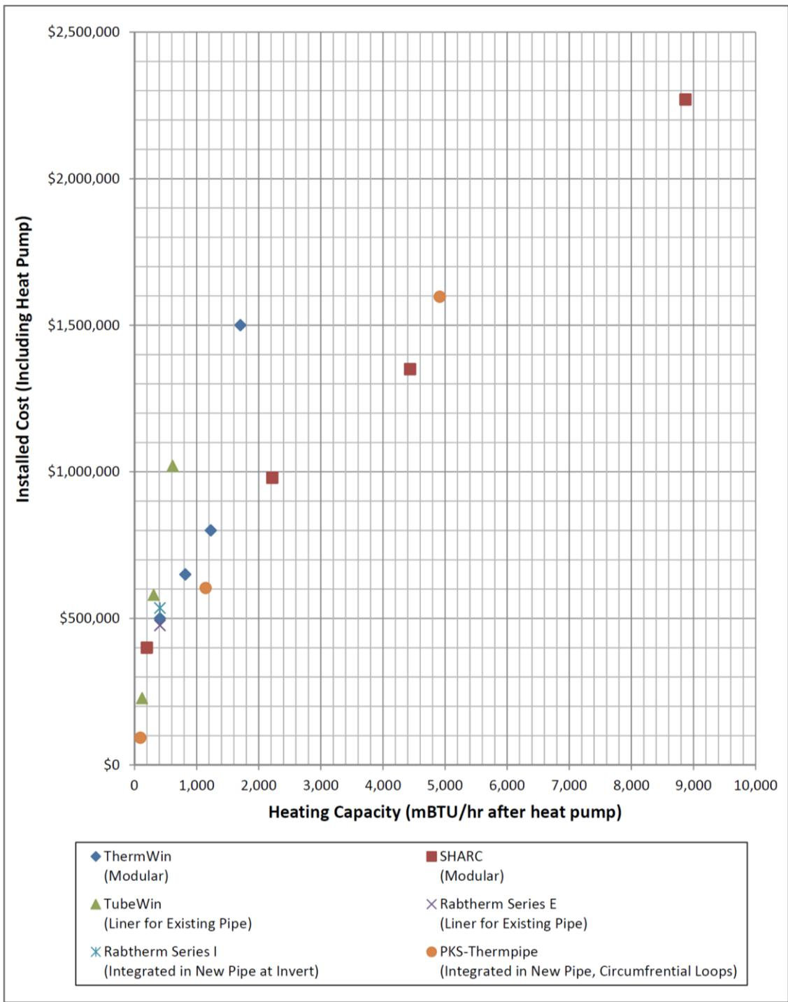
Figure 15. Sewer Heat Recovery Installed Cost Vs. Heating Capacity.<sup>26</sup>
