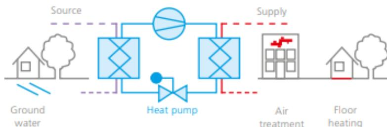
Figure 1. Heat Pump Flow Diagram.
