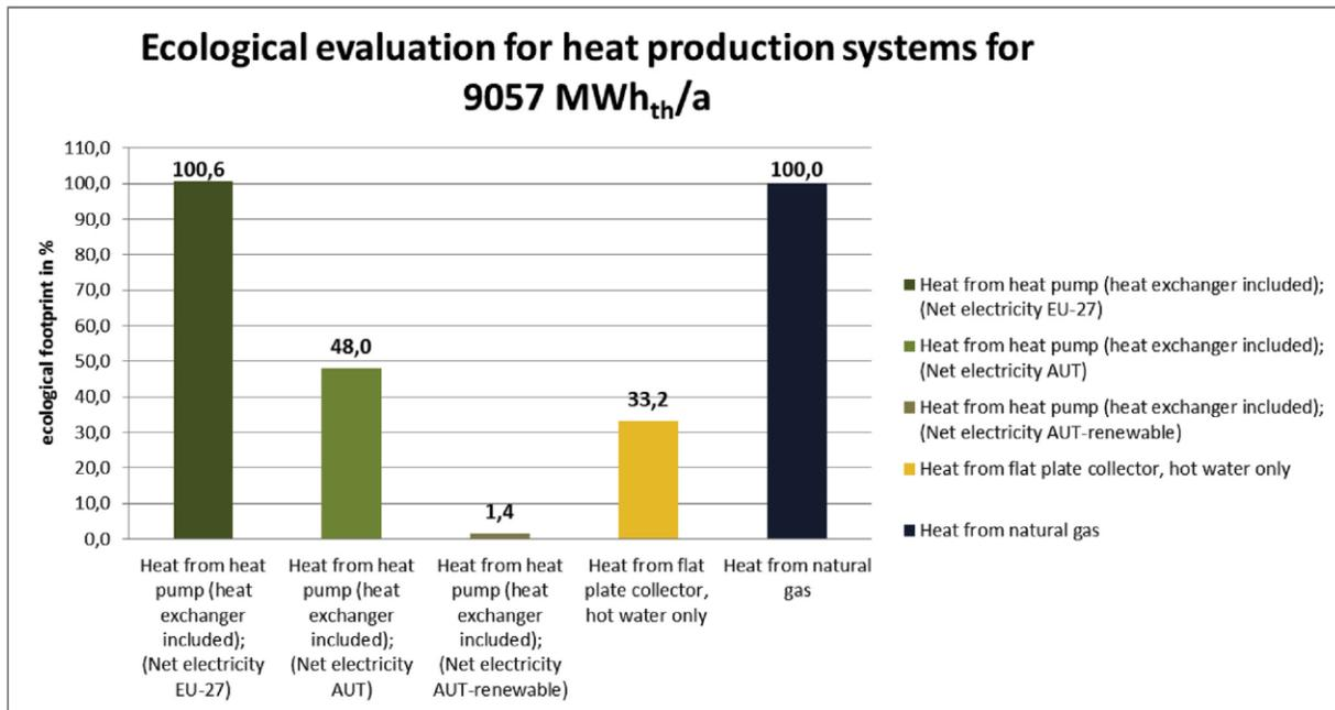
Figure 5. Ecological Evaluation of the Heat Production System in Freistadt WWTP.<sup>14</sup>
