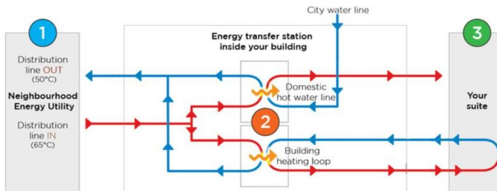
Figure 3. District Energy Layout with a Transfer Station for Heating.<sup>5</sup>
