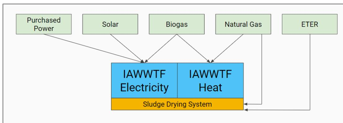
*Figure 20.* Sources and Uses of Heat in IAWWTF.
