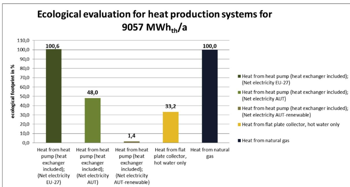
Figure 5. Ecological Evaluation of the Heat Production System in Freistadt WWTP.<sup>14</sup>
