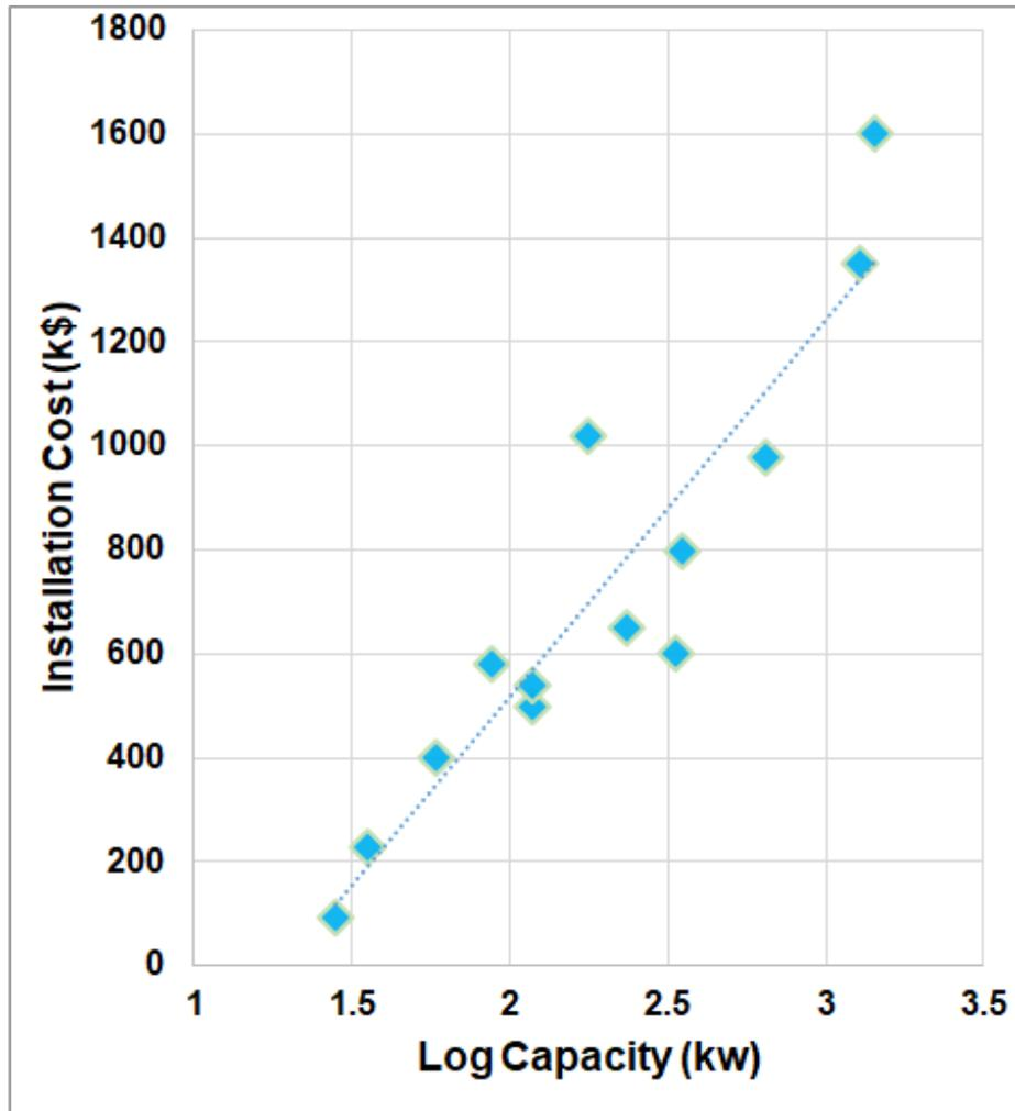
Figure 16. Logarithmic Model of Installation Cost (\$000) Vs. Log Capacity (kW).
