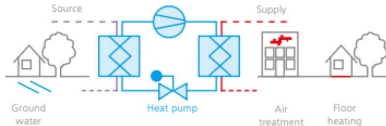
Figure 1. Heat Pump Flow Diagram.
